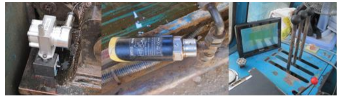
Figure 11 Wire spring penetration decoder, pressure transducers at the hydraulic system and LCD panel at the operator cabin
