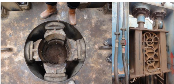
Figure 3 Hydraulic gripping system with gripping blocks
