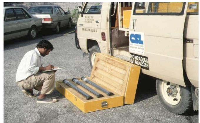
Plate 2 Sample protection and transportation as practised by CSL
