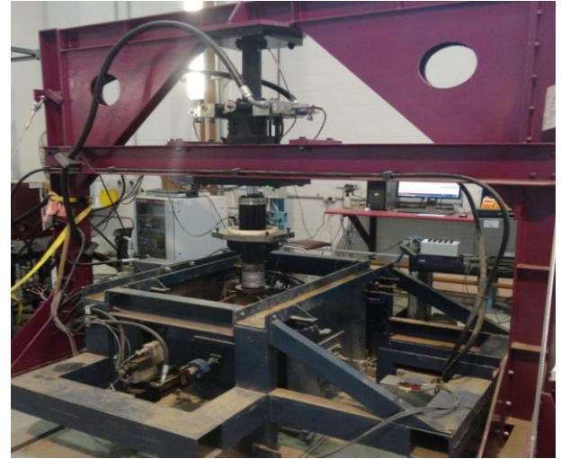
Figure 7(a) Process Simulation Prismoidal Triaxial Apparatus (PSPTA) designed and built at University of Wollongong
