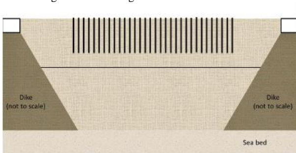
Figure 16 Use of short PVDs and vacuum preloading to form a working platform
