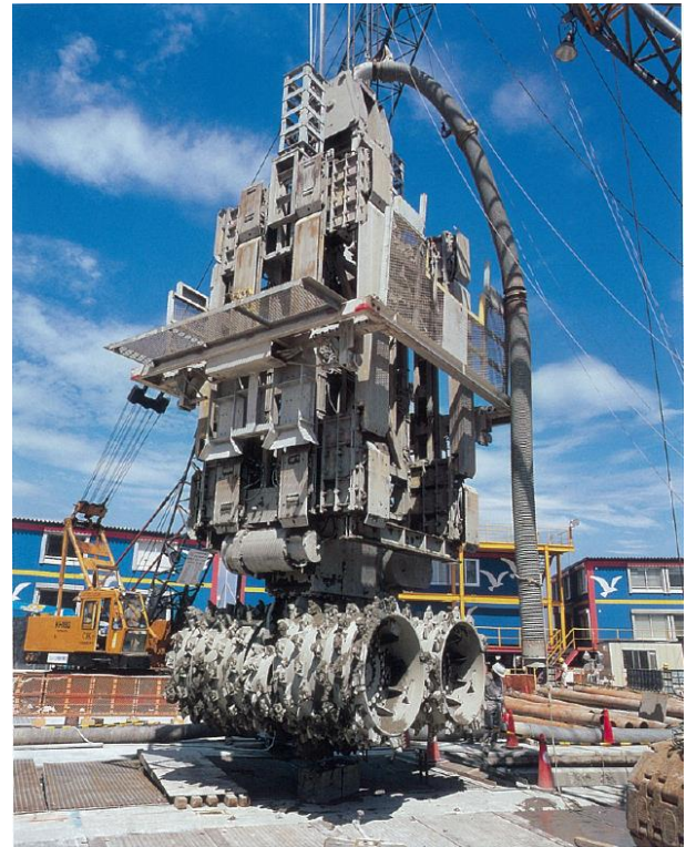
Figure 49 Two-axes rotating type cutting bits
