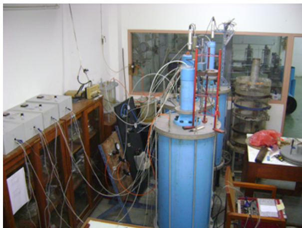
Figure 1 Large scale consolidometers for Thermal PVD and Thermal Vacuum PVD
