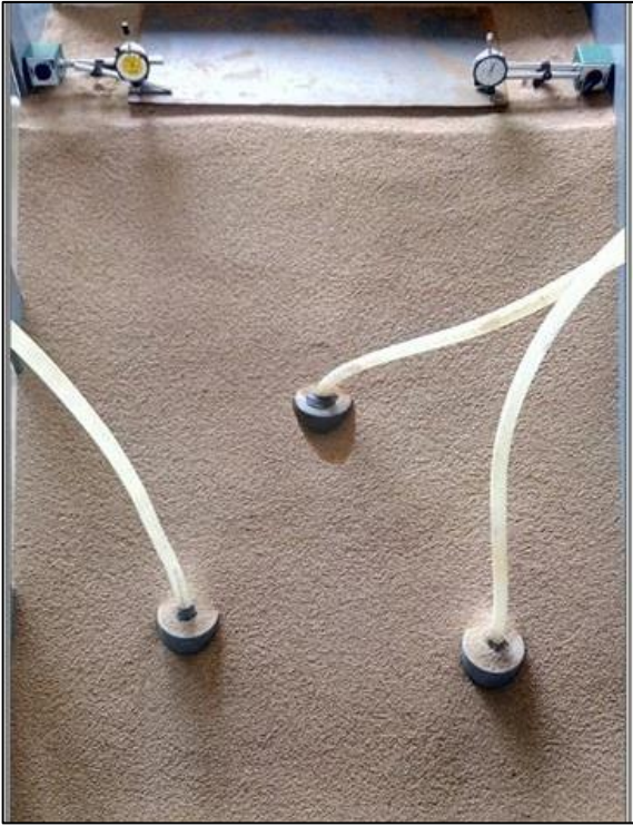
Figure 5 Slope incorporated with sand drains and dial gauges
