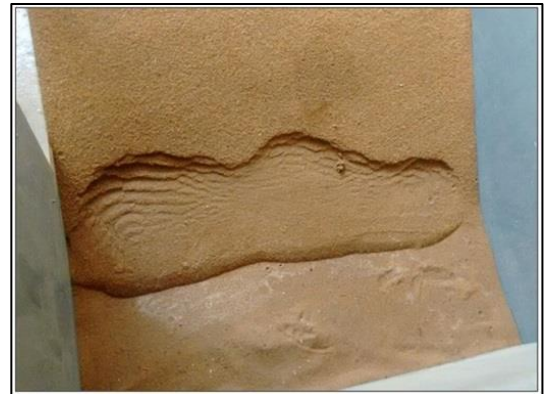
Figure 8 Slope Failure Pattern
