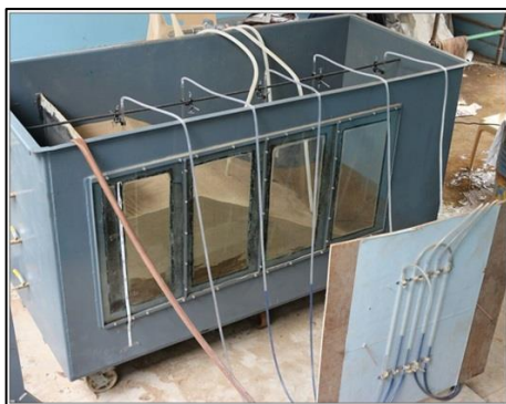
Figure 1 Tank and Manometer Setup
