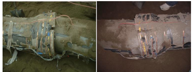
Figure 9 Examples of pipeline joints crushed during the first test
