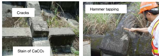
Figure 7 Visual inspection and hammer tapping on the concrete cap of anchor
