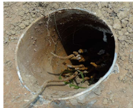
Figure 2 Seriously corroded and broken steel strands found from at the landslide site
