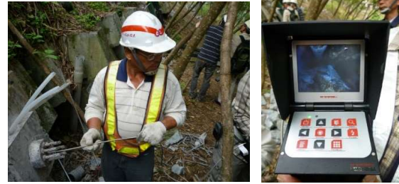
Figure 9 Use endoscope to inspect steel strands under anchor head
