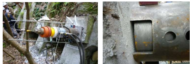
Figure 10 Lift off test for determining the residual anchor load
