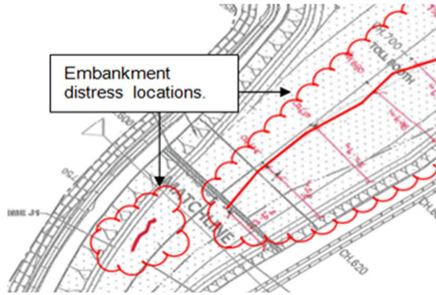
Figure 3 Layout Plan of embankment distress
