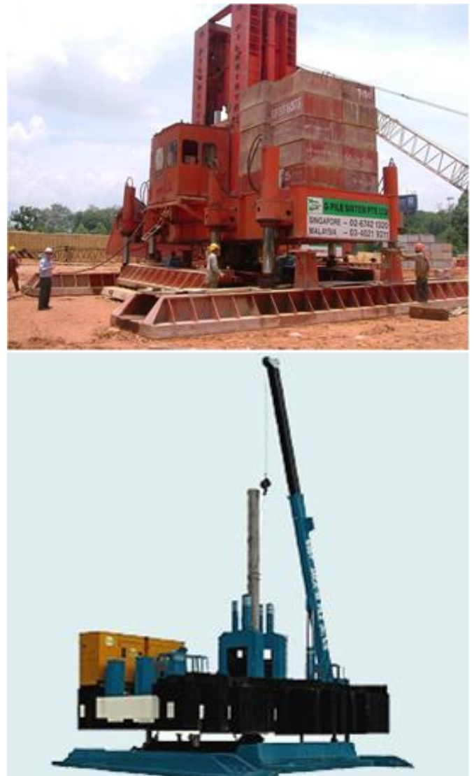
Figure 1 Typical high capacity jack-in pile machine in Malaysia
