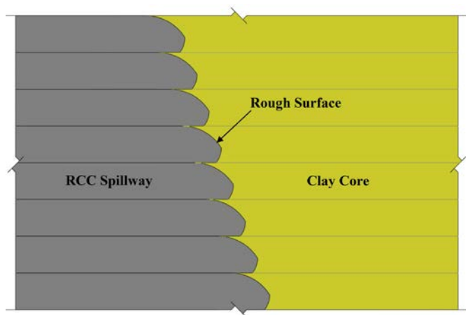
Figure 32 Rough surface between RCC spillway and clay core
