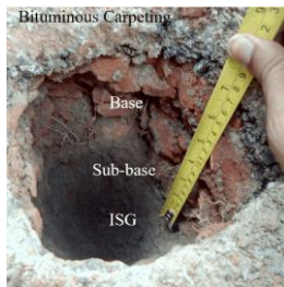
Figure 31 Verification of pavement layer thicknesses by making a hole on road pavement.
