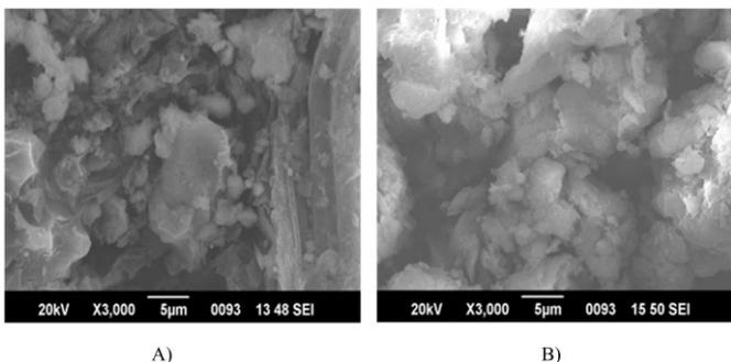
Figure 9 SEM marine clay (A) Untreated, (B) Treated
