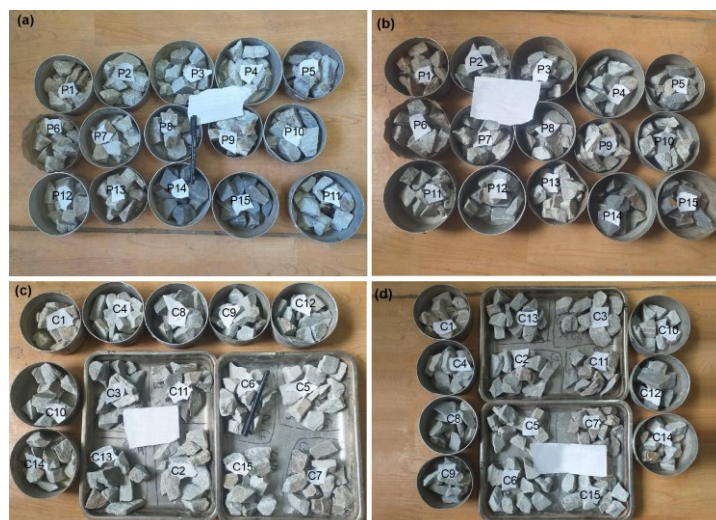
Figure 6 Samples under slake durability test showing type I deterioration. (a) samples from the Pandrang Quartzite after the second cycle, samples from the Pandrang Quartzite after the fifth cycle, (c) samples from the Chisapani Quartzite after the second cycle, and (d) samples from the Chisapani Quartzite after the fifth cycle
