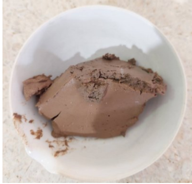
Figure 1 Bentonite sludge after being treated with polymer
