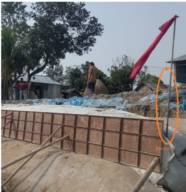
Figure 14 Steel bar used to measure settlement of the embankment
