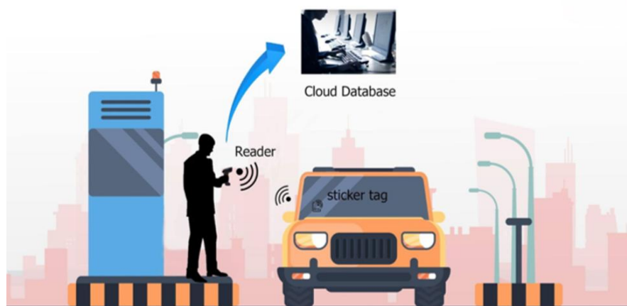
Figure 1. System architecture of the proposed RFID-driven smart border passing system.
