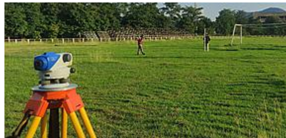
Figure 12 Leveling procedure using an automatic level
