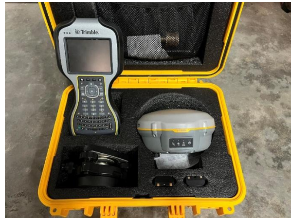
Figure 7 GNSS receiver Trimble R8s and supporting accessories
