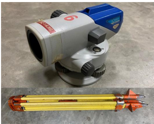
Figure 5 Leveling instrument: Sokkia C31 with tripod.
