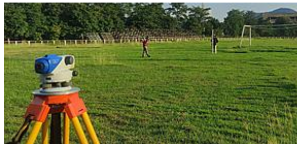
Figure 12 Leveling procedure using an automatic level
