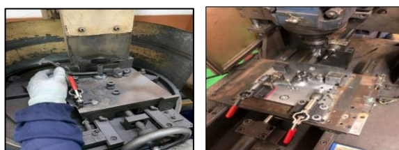
Before After Figure 11 Before and after Jig Fixture implementation
