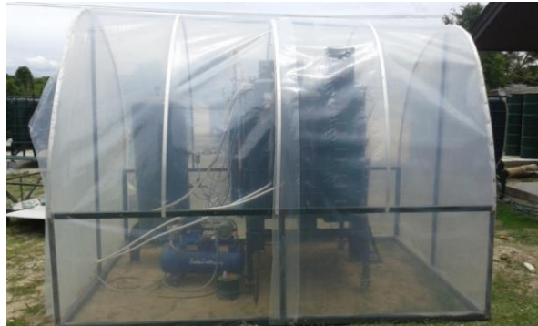
Figure 4 Solar greenhouse covering the entire 1,000 L biogas digester system
