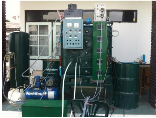
Figure 2 The 1,000 L biogas production system
