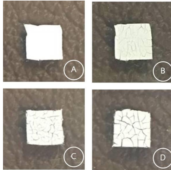
Figure 7 The ZnO surface structures when coated with (a) 1 layer, (b) 2 layers, (c) 3 layers and (d) 4 layers.
