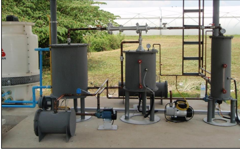
Figure 17 A full scale solar driven 2 tons single stage ejector refrigeration experimental system
