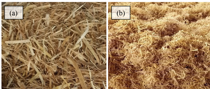
Figure 1 Characteristic of corn husk (a) Smaller particle size by a grinder (b) Corn husk fiber after pretreatment with 10% NaOH solution
