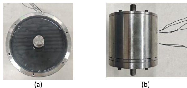
Fig. 21 (a) MR mount prototype after MRF injection (b) MR mount prototype.
