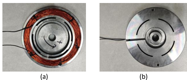
Fig. 18 Flow mode coils winding and compaction: (a) the flow mode coils and (b) install the partition.
