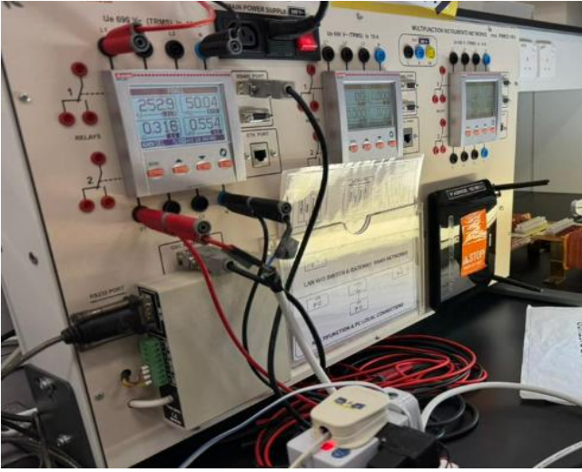
Fig. 8 Measurement setup showing DDEMS validation against Lovato DMG800 power multimeter.
