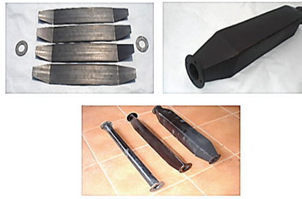
Figure 4. Heat duct design (a) Circular cross-sectional duct (b) Square cross-sectional duct and (c) Triangular cross-sectional duct.
