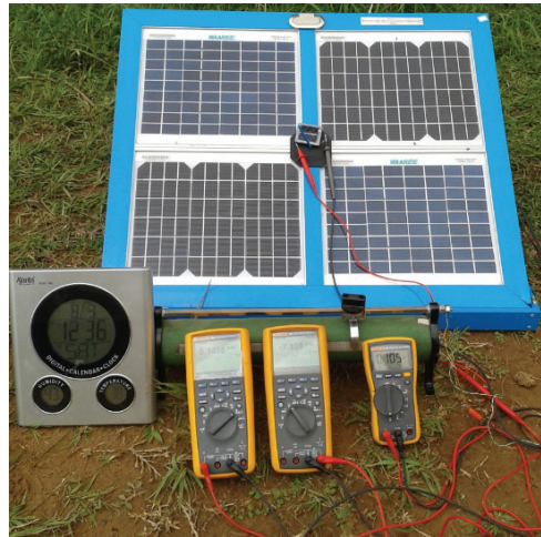
Figure 1 PV module measuring set up
