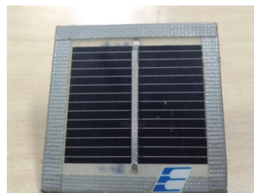
Figure 2 Calibrated solar cell
