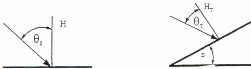
Fig. 2 The solar radiation incident on a planar surface and an inclined plane
