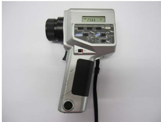
Fig.3 Surface Brightness Checking Instrument
