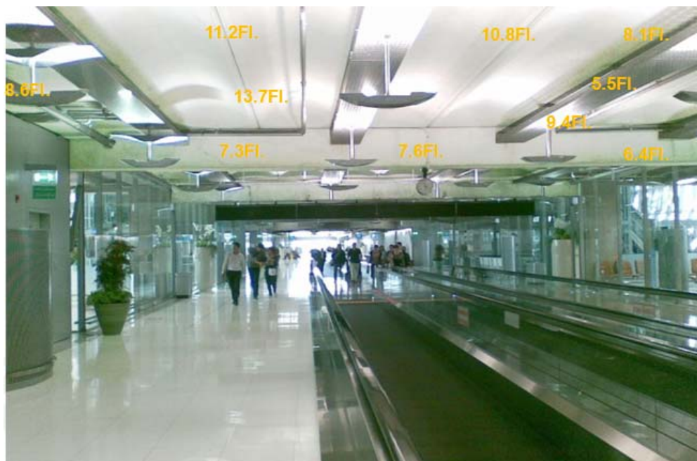
Fig.12 The surface and ceiling brightness after studying
