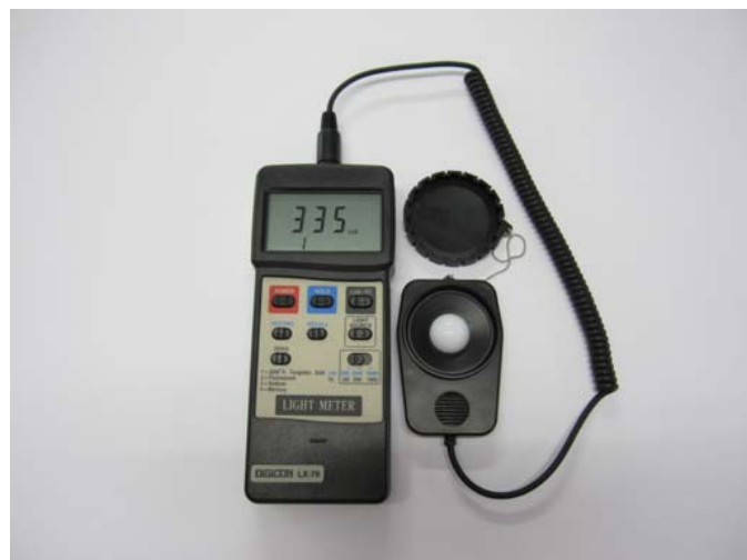
Fig.2 Brightness Checking Instrument
