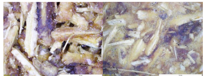
Fig. 5 Light microscopic observation at a magnification of 3x of the 1:4 sunflower stalks and natural latex bio-composite obtained using a hot oven (left) and the 1:6 sunflower bark and natural latex bio-composite obtained by hot compression (right). The scale refers to 10 mm.
