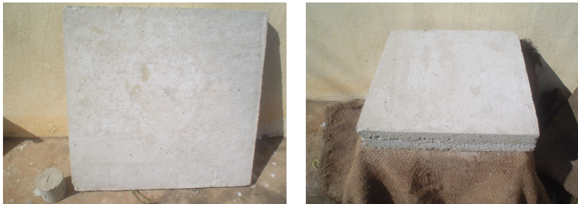
Fig. 2 Configuration of tested sample of concrete mix materials with the size of 30 cm.*30 cm*2.54 cm.
