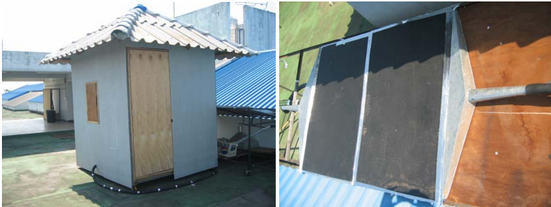
Fig. 1 (a) The house model used in the experiments (b) The Area changeable sky radiator
