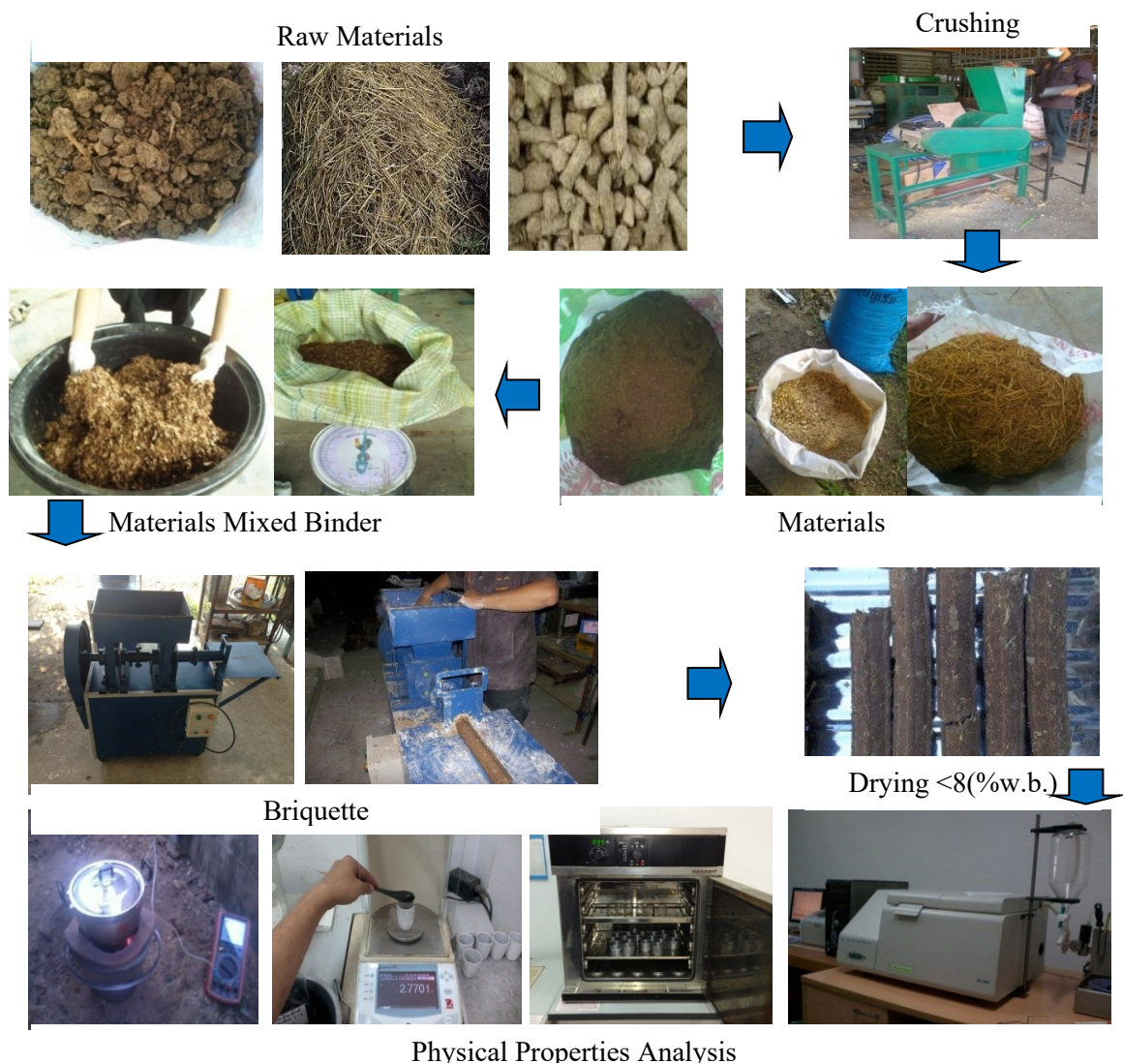
Fig. 2 The production of fuel briquettes.
