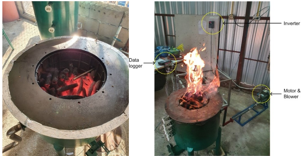
Fig. 2 The biomass stove experimental setup.
