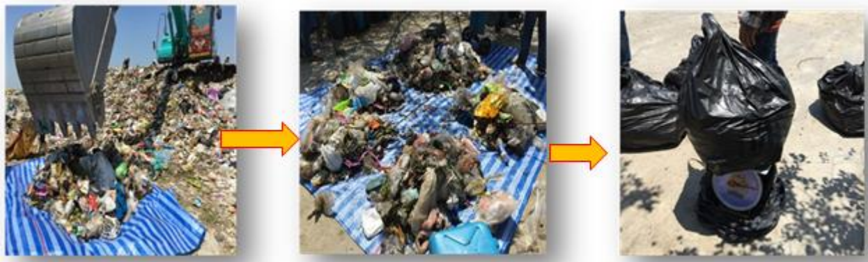
Figure 2 MSW in experiment collected from Nonthaburi Provincial administration Organizations by quartering method.
