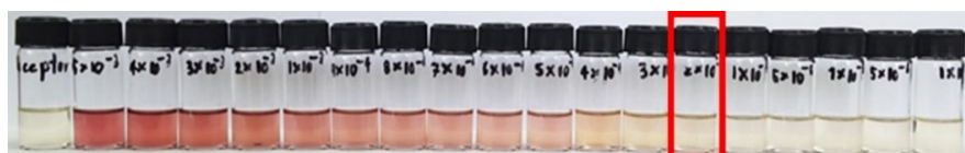
Figure 4 Color changes of S1 ( 5 \times 10^{-5} M) in acetone with various concentrations of CN - .
