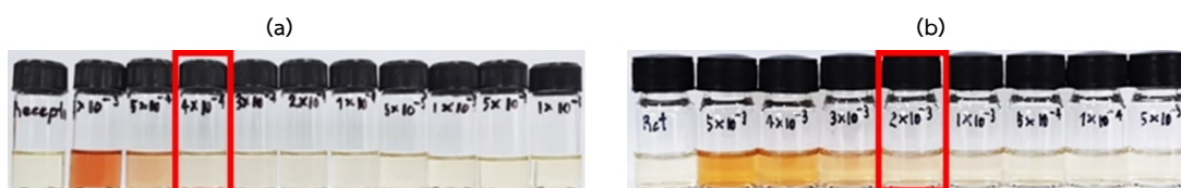
Figure 5 Color changes of S1 ( 5 \times 10^{-5} M) with various concentrations of (a) F - in acetone and (b) F - in acetonitrile: acetone (7:3).
