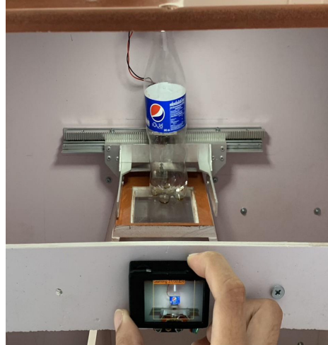
Figure 2 The Huskylens IDE program for object recognition and identification
