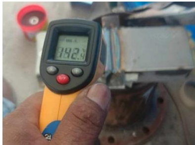
Figure 9 Measuring temperature on the surface of the workpiece with an infrared thermometer
