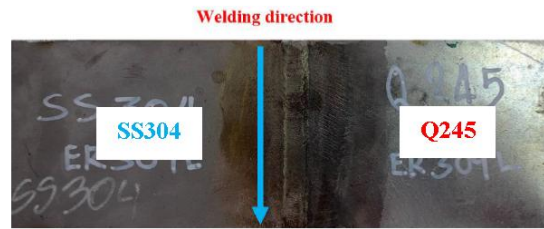
Figure 1 The specimens of SS304 and Q245 welded by gas tungsten arc (GTAW) method
