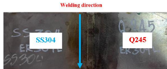
Figure 1 The specimens of SS304 and Q245 welded by gas tungsten arc (GTAW) method
