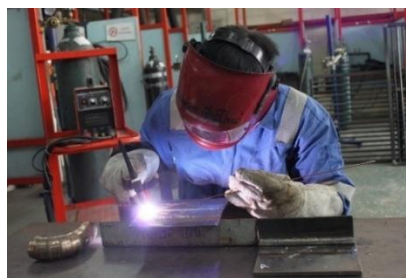
Figure 2 Gas tungsten arc welding process (GTAW)
