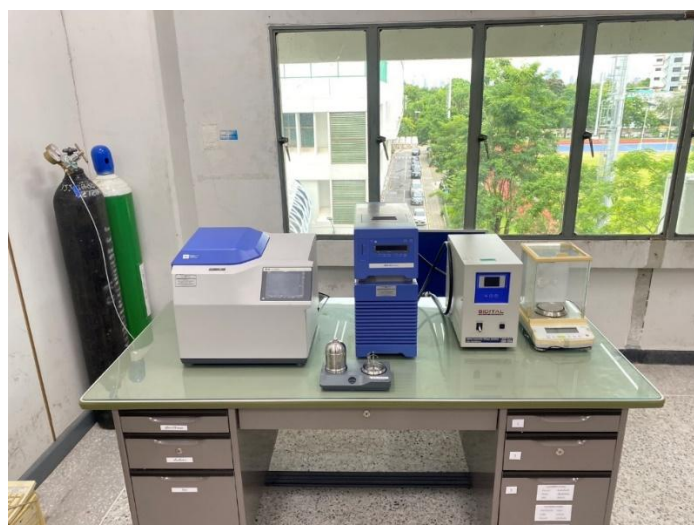
Figure 2. Bomb Calorimeter used in laboratory instruction.
