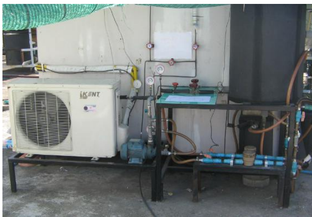
Figure 5 Condensing Unit, Pressure gage, Control Valve and Hot Water Tank.[7]
