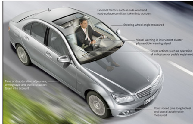
Figure 16 How the Tired Drivers System from Mercedes works [30].
