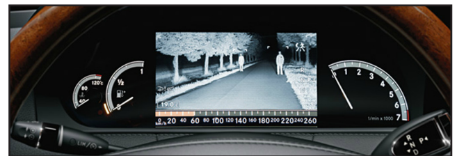
Figure 14 The infrared night view system on Mercedes-Benz CL-Class [25].
