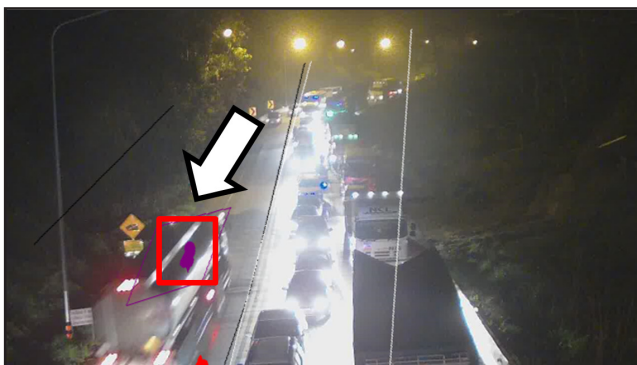
Figure 16. The error of reflection between moving truck and traffic sign
