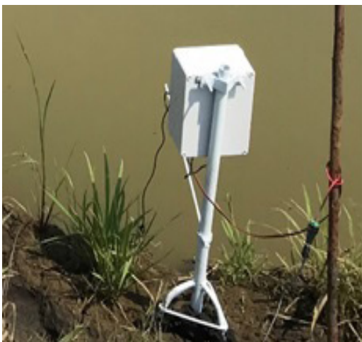
Figure 2. Devices setup in the testing site with a locked cover to prevent hazard and accident from surrounding.
