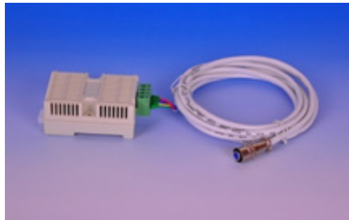
Figure 3. The IC sensor number SHT10 encased with the plastic container.
