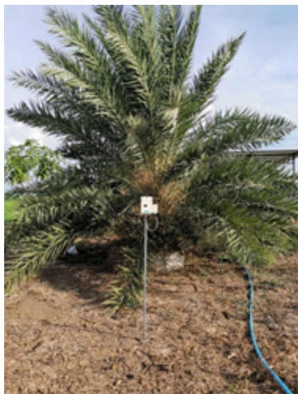
Figure 9. The ambient sensor-node deployed in the crop area.
