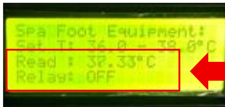
Figure 7: LED Display of the foot spa machine operation when the temperature exceeds 37 °C
