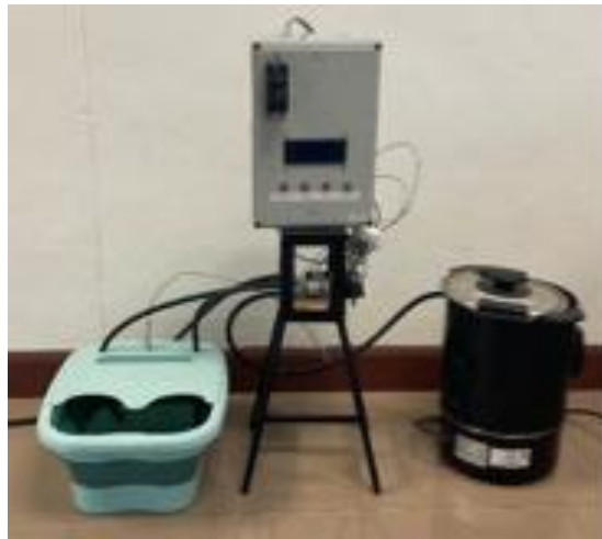
Figure 4: Installation of the temperature control system inside the foot spa basin
