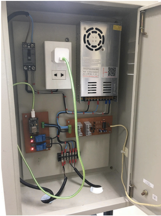
Figure 5. The control circuit of the chicken feeder machine.
