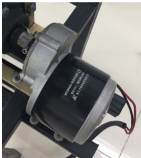
Figure 4. DC gear motor 24 V 350 W.
