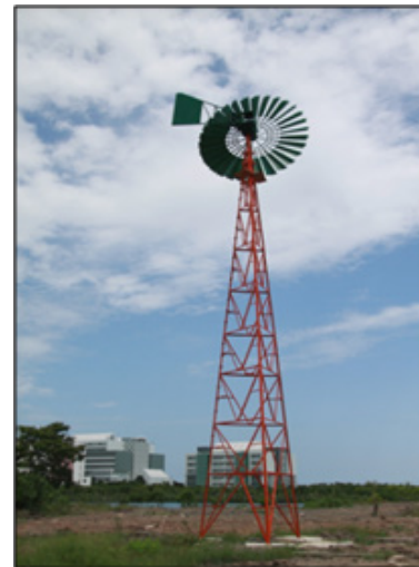
Figure 1(d). Multi-blade wind turbine in operation
